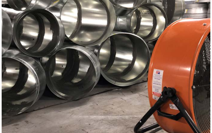
Spiral Pipe of Texas (SPOT) sealed duct with forced air curing
