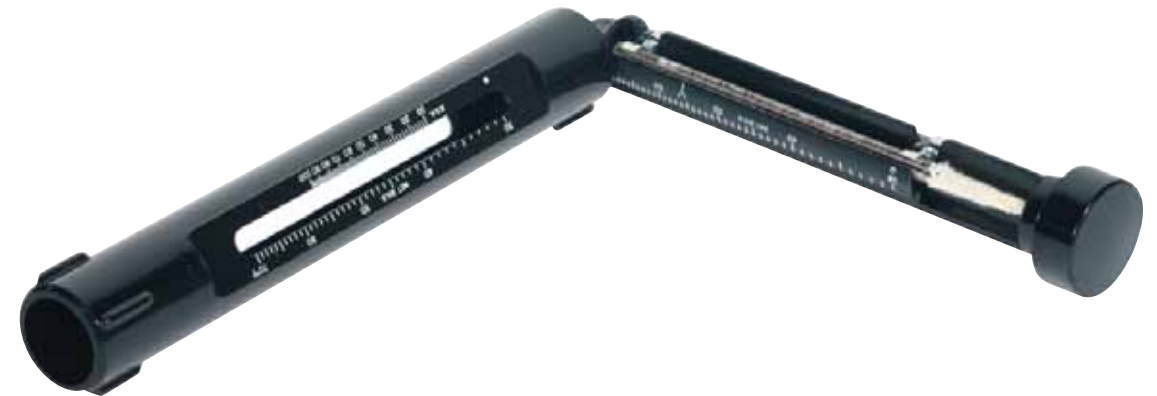
Figure 1 (left). This is a photo of a cabinet door that is showing shrinkage due to low humidity. (Photo by Bill Johnson) Figure 2 (above). A sling psychrometer uses the wet-bulb/dry-bulb principle to provide humidity readings. (From Refrigeration & Air Conditioning Technology, 5th Edition, by William Whitman, William Johnson, and John Tomczyk, published by Delmar Cengage Learning.) (©Delmar Cengage Learning.)
