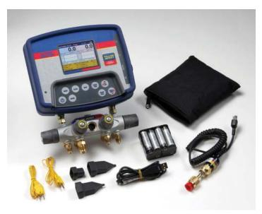
The YELLOW JACKET® refrigeration system analyzer comes in a blow-molded carrying case complete with a TITAN<sup>TM</sup> 4-valve test and charging manifold, vacuum sensor cordset, battery holder ('AA' Size, 2X4), instrument boot, bumper, plug, and sensor/probe boots, USB cable, vacuum sensor and two general purpose "K-Type" probes.
