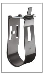
The spring steel hanger grips the rod tightly, and the black zinc coating offers corrosion resistance while matching the insulation color. The clamp can be detached from the rod hanger and used to secure lines to flat surfaces (see photo at right).
