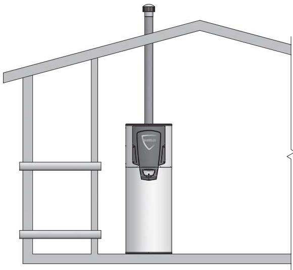
Figure 1-4_Combustion Air Through Ducts
