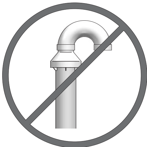
Figure 4-5 Do Not Install U-Bent to Rain Cap
